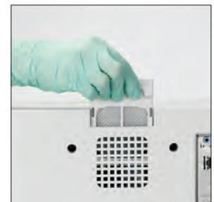
10. Remove the fan filter, rinse it thoroughly with warm water, pat it dry with a paper towel, and return it to its location in the analyzer. Then on the SediVue Dx Cleaning Guide screen, tap **Done** to power on the SediVue Dx.
