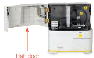
**Note:** Do not open the analyzer door while a run is in progress as it will cancel the run and discard the sample and cartridge.
